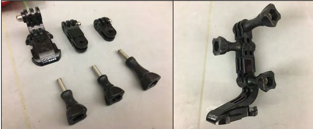
Figure 2. Go Pro attachment gear to hold cameras onto the PVC structure.
