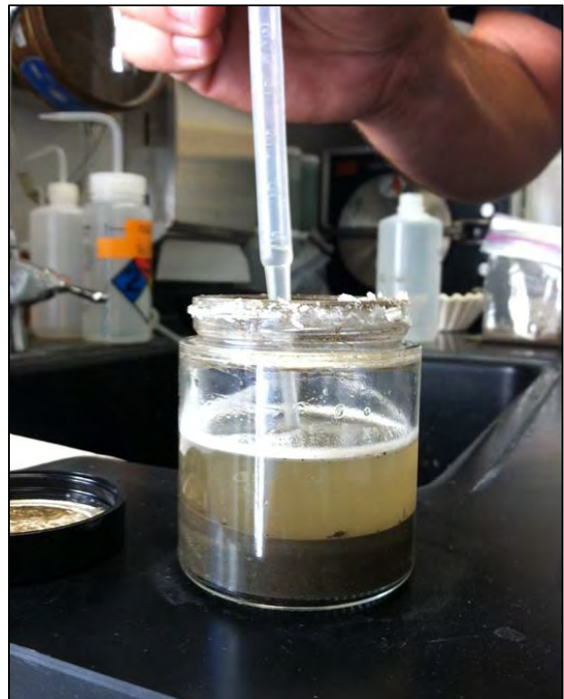
Figure 4. Eyedropper collecting water to test salinity.
