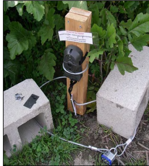
Figure 3. Motion activated wildlife camera secured to cinder blocks and a 2 x 4” stake.
