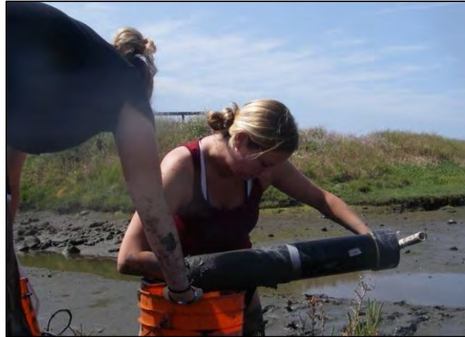
Figure 3. Example of large core sediment extraction.
