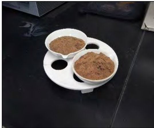
Figure 6. Hot crucibles placed on crucible stand.
