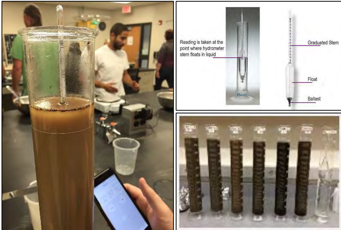
Figure 9. Hydrometer floating in a 1000 ml cylinder (left), diagram of how to read hydrometer (top right) from Amazon.com), and 1000 ml cylinders with sediment and sodium hydroxide (bottom right).
