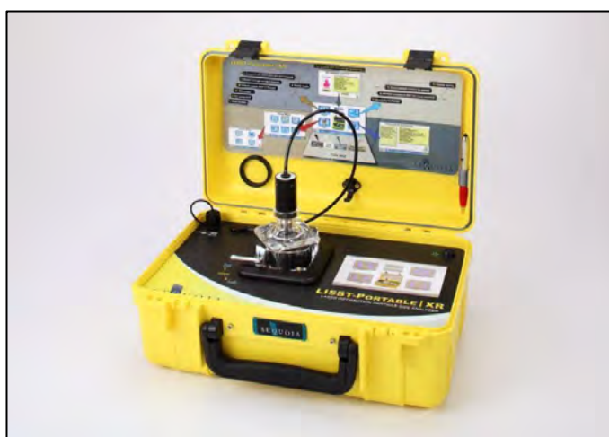
Figure 1. LISST-Portable Laser Diffraction Par (courtesy Sequoia Scientific).
