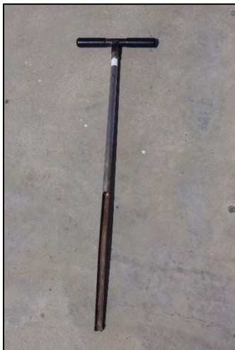
Figure 2b. Soil corer.
