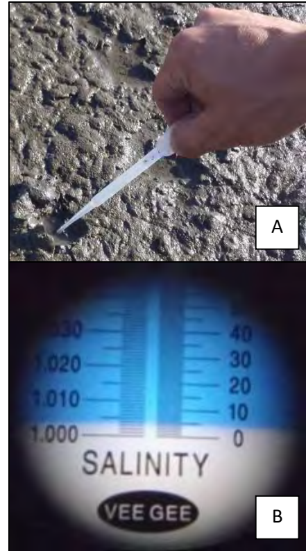
Figure 3. Eyedropper removing pore water from a shallow depression (A) and reading the refractometer (B).
