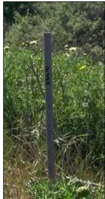
Figure 3. UV-resistant PVC pipe marking the beginning of a vegetation transect.
