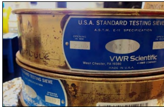
Figure 4. Stacked sieves of decreasing screen size.
