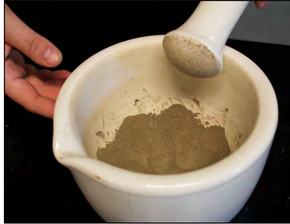
Figure 4. Homogenized sediment sample with mortar and pestle.
