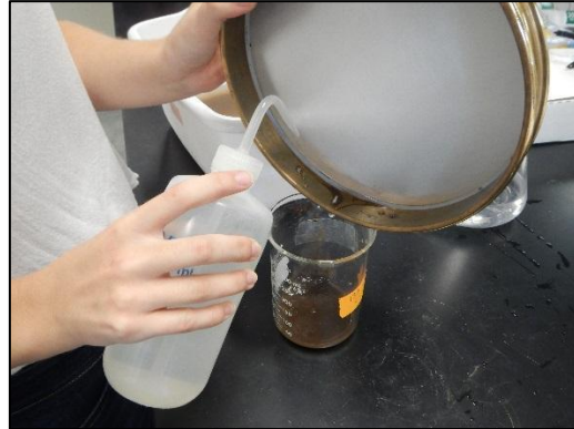
Figure 7. Rinsing sediment from sieve.
