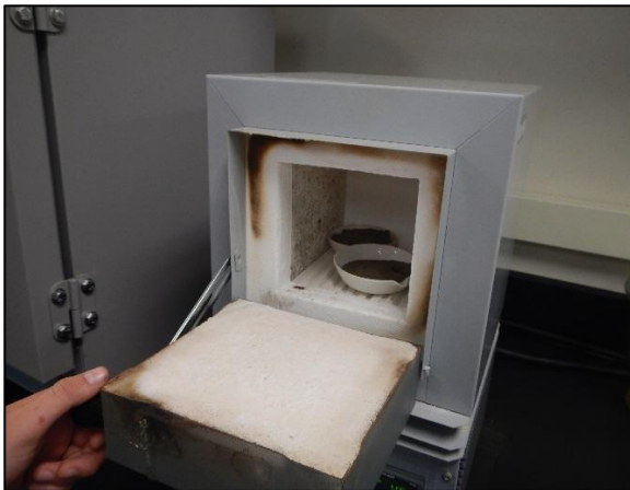
Figure 5. Place crucible carefully in furnace.
