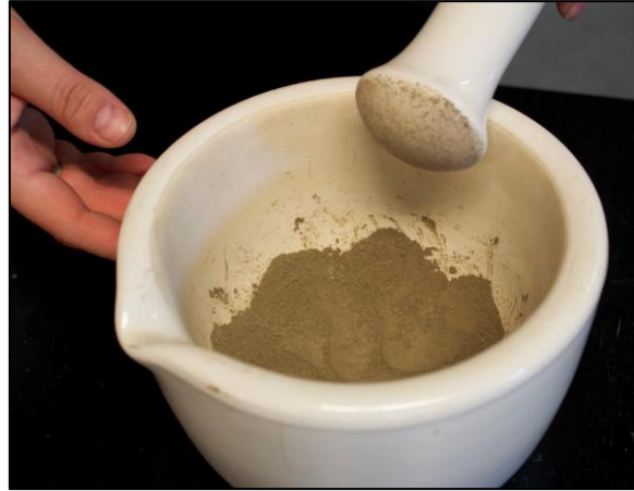
Figure 4. Homogenized sediment sample with mortar and pestle.
