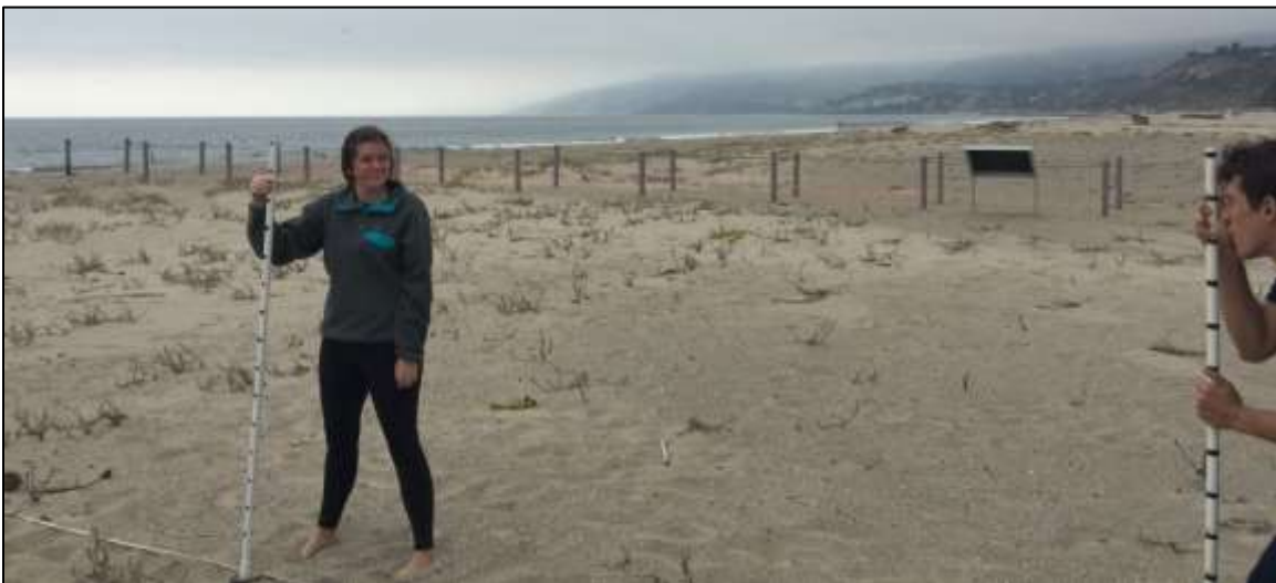
Figure 25. TBF staff and CRI interns conducting an elevation profile survey on 6 November 2019.
