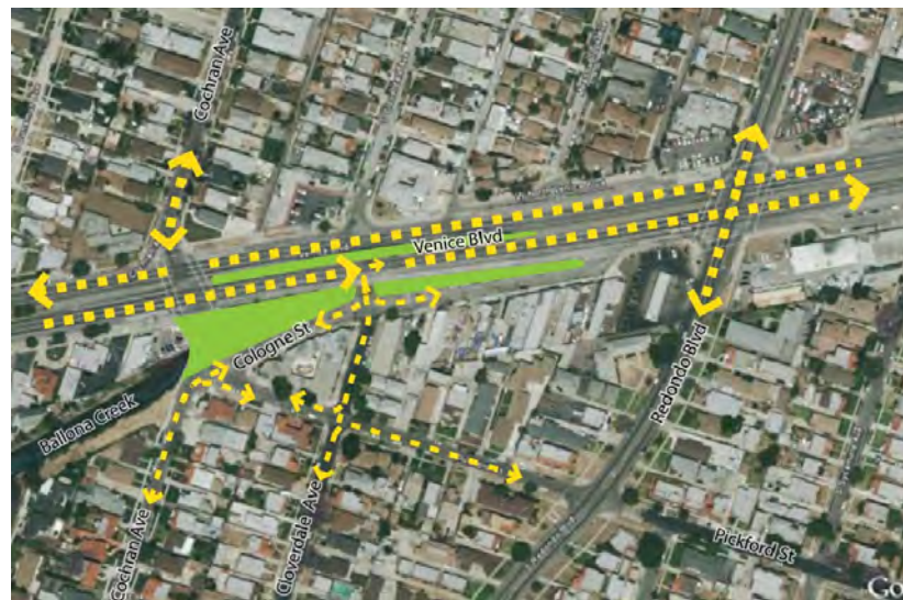
Figure 2. Potential traffic conditions if Cochran Avenue is closed at Venice Boulevard and Cloverdale Avenue is extended north Venice Boulevard.
